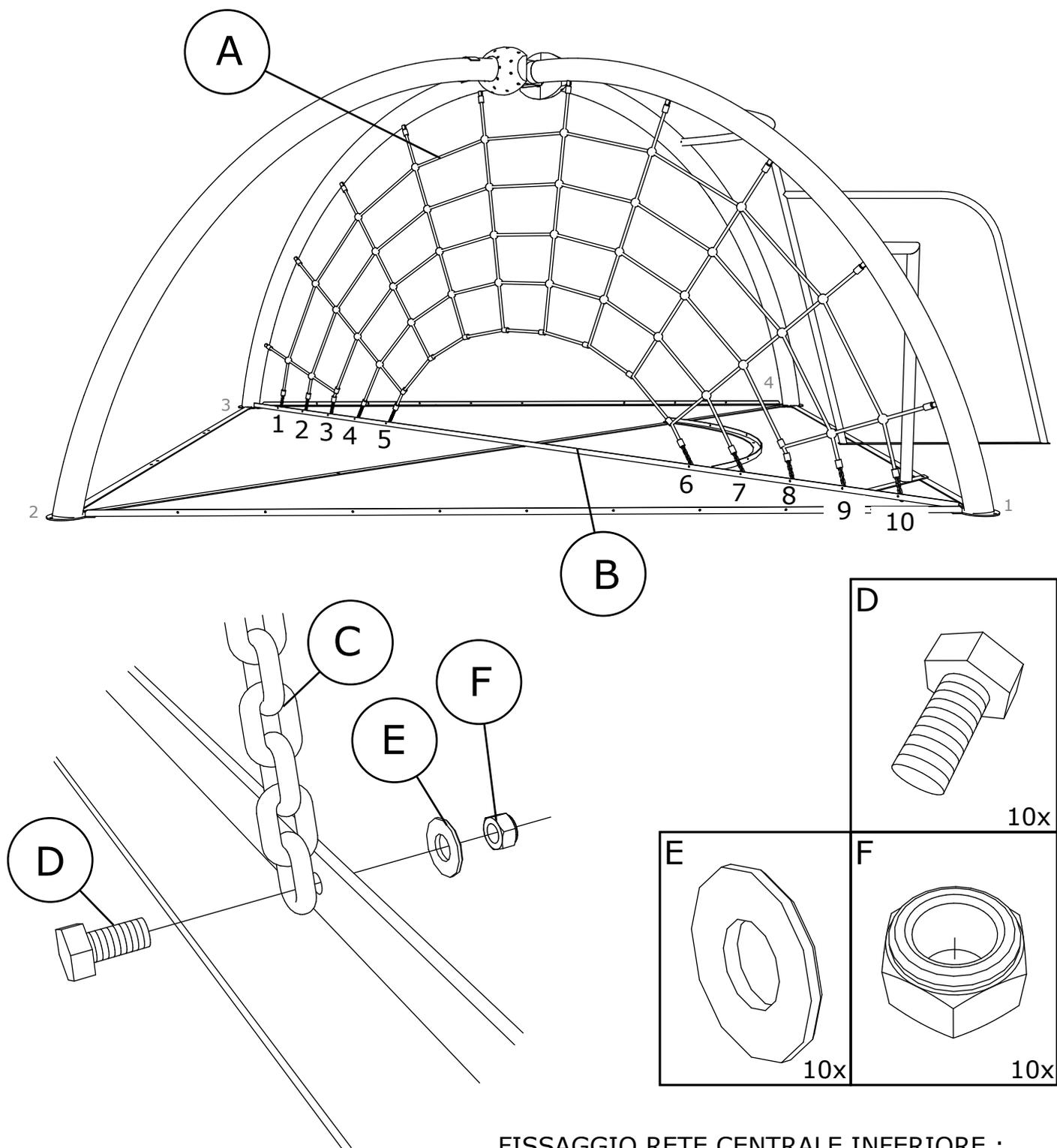
**FISSAGGIO RETE CENTRALE INFERIORE :**
